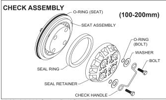
All Model 310 Series Backflow Preventers must be inspected and maintained by an accredited backflow prevention tester at least once a year or more frequently as specified by local codes. Replacement of worn or damaged parts must only be made with genuine "ZURN WILKINS" parts.
