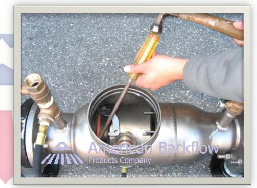
Tap with hammer in counterclockwise direction to loosen.
